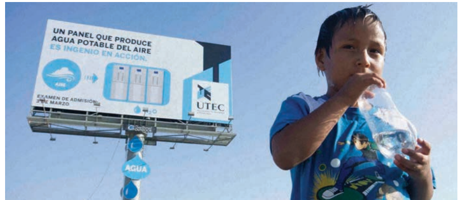
Billboard in Lima, Peru that converts very humid air into clean drinking water for residents.
